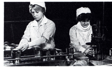
The operator on left is shown applying lids as cans pass down line, and the second operator is placing cans under lid compressor.
