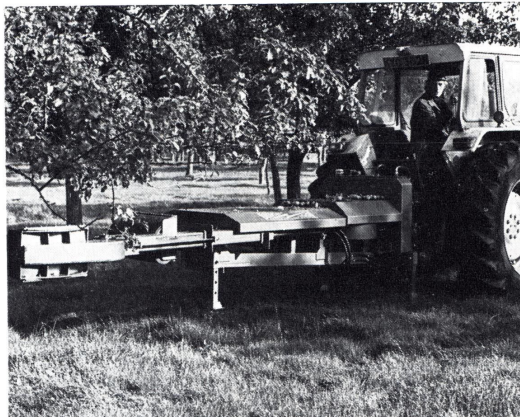
The Lightning Tree Shaker, now used on five of the six fruit units, can shake 100 trees an hour in the hands of a skilled operator.
