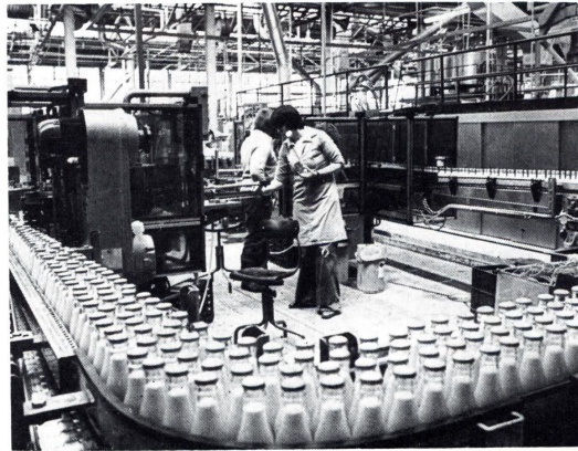
A Kronos Cronomatic Type 55 labelling machine being replenished without interrupting the flow of bottles.
