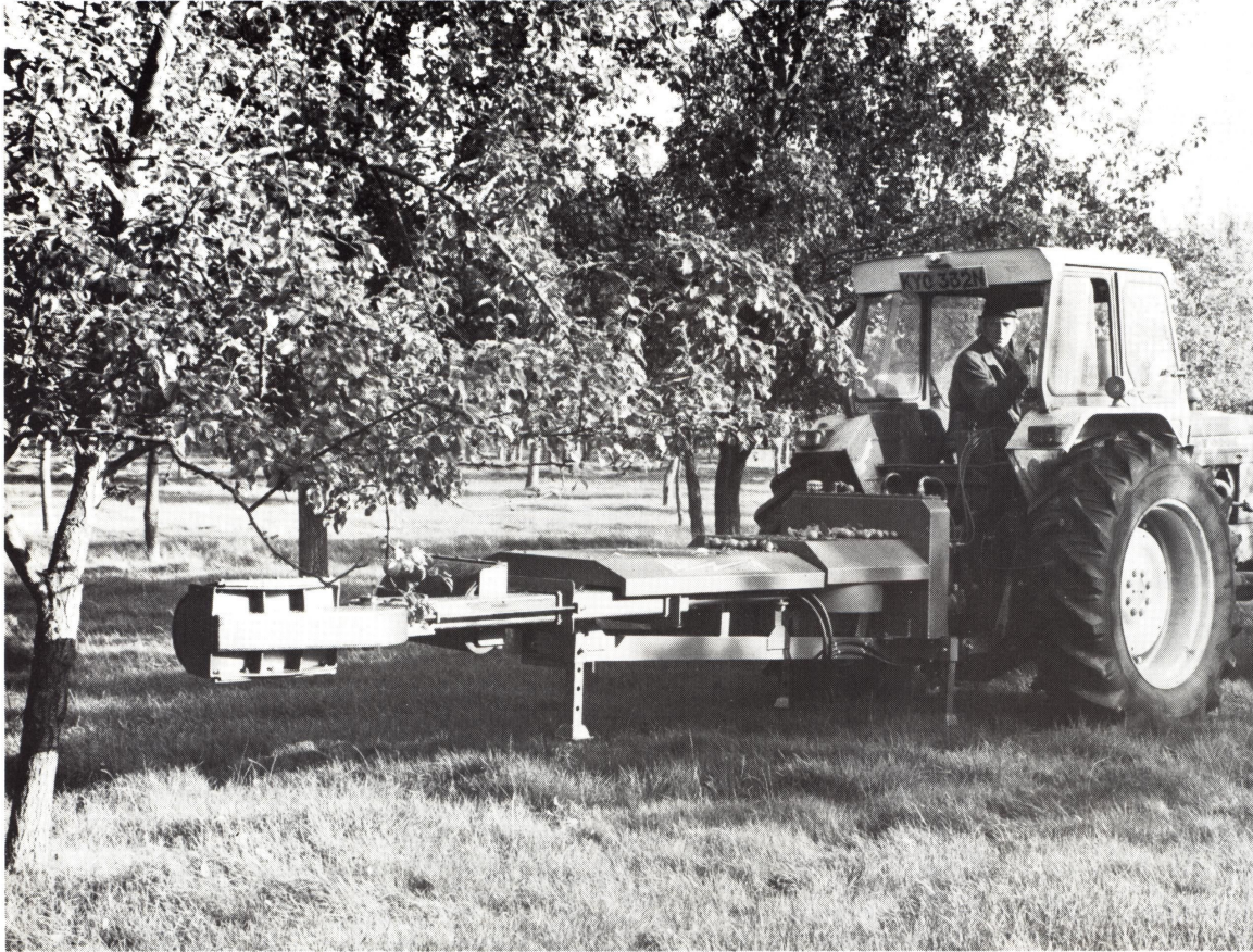
Operator Aubrey Sellick backs a Lightning Tree Shaker onto a perry pear tree at Middle Chipley Farm, Somerset, during Autumn Harvesting.
