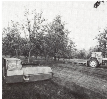
Two items of modern machinery in use at Middle Chipley Farm, Somerset: A harvester (left) moves along scooping up the pears shaken from the trees by the shaker (right).
