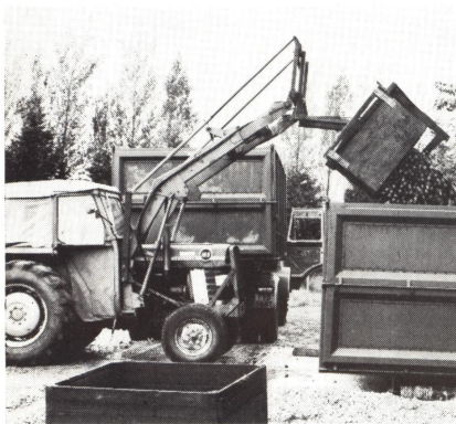
A bin tipper at Middle Chipley Farm, Somerset releasing a bulk bin of perry pears ready for transporting to Shepton Mallet, where Babycham sparkling perry will be produced from them.
