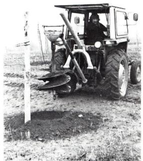
No hard work these days! Eric Wadham, tractor driver on Showerings' Yard Farm, Bishops Lydeard, Somerset, demonstrates the efficiency of a Danuser post hole borer in digging tree planting holes.
