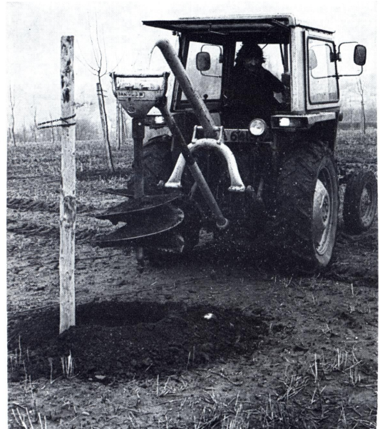
No hard work these days! tractor driver on Showerings Yard Farm, Bishops Lydeard, Somerset, demonstrates the efficiency of a Danuser post hole borer in digging tree planting holes.
